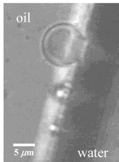
Figure 4. Contour of a pendant water drop after injection into a dodecane suspension containing 0.25 mg/mL POPC. This image shows the presence of droplets at the dodecane–water interface. The fact that the droplets grow into the dodecane confirms that the spontaneous formation of droplets happens at the interface.
