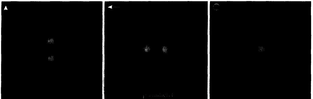
Fig. 7. Simulation of fluorescence images of single molecules. The molecules are located on a transverse plane below the tip shown in Fig. 5b. The orientations of the transition dipoles are indicated by the arrows. A tip sample separation of 2 nm is assumed. The patterns of the horizontal dipoles are amplified by a factor of 5.
