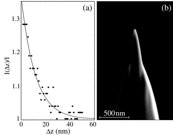
FIG. 3. (a) Dependence of the Raman scattering strength of the  $G'$  band ( $I$ ) on the longitudinal separation ( $\Delta z$ ) between a single SWNT and the tip. The solid line is an exponential fit with a decay length of 11 nm. The signal is normalized with the far-field signal. (b) Scanning electron micrograph of a sharp silver tip fabricated by focused ion beam milling.
