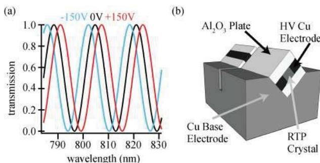
Fig. 2. (a) Schematic modulator transmission versus wavelength for three applied voltages, calculated using the  $50\lambda$  plate at 800 nm and the 2-mm-thick modulator crystals. (b) Modulator layout, showing thin RTP crystals with perpendicular orientation, sapphire ( $\text{Al}_2\text{O}_3$ ) plates to minimize thermal gradients, and the copper (Cu) ground and high voltage (HV) electrodes.
